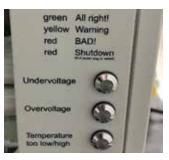
The HY-115 Pump is equipped with three-colored (3) LED lights integrated into the electric control box for system monitoring. The LED lights let you know that you are operating within voltage and temperature limits.
