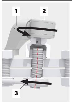
Torque wrench and backup wrench rotate in same direction.
