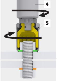
The HYTORC Washer grips surface while the backup washer keeps the bolt in place and square with the surface.
