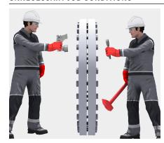
Pinch hazards and more personnel; damaging side loads; bending forces; shorter lifespan of nuts and bolts.
