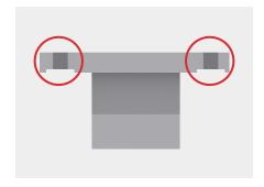
Repeated tightening and loosening of nuts and bolts cause extended wear and damage (re-machining) to flange surfaces.
