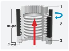
The HYTORC Nut is composed of an inner sleeve (1), outer sleeve (2), and washer (3). As the outer sleeve turns (blue arrow), the inner sleeve moves upwards (red arrow). The washer spline rotationally couples the inner sleeve with the washer preventing the inner sleeve from turning while providing a solid reaction point for turning the outer sleeve.
