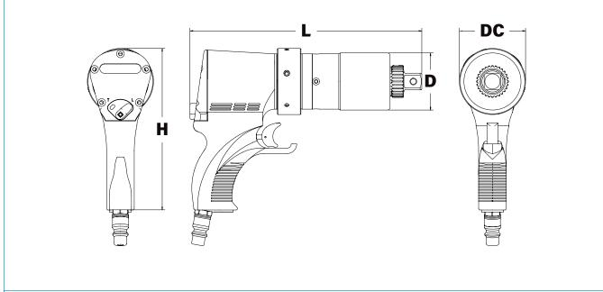
LEGEND: H = HEIGHT L = LENGTH D = OUTER DIAMETER OF GEARBOX DC = DIAMETER OF COLLAR
