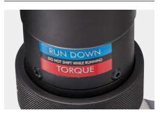
A simple twist of the collar switches the tool from high speed rundown mode into the max power mode with adjustable torque so you can choose the right output for your job.
